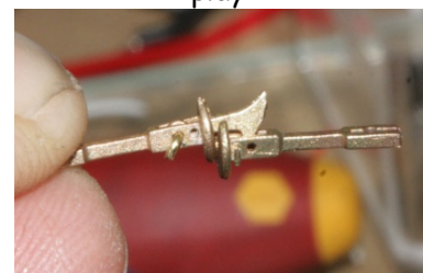
Check to see locking action works
