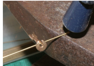
Peen the end of the wire
