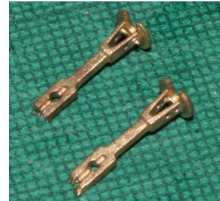
Remove a pair of heads from the sprue, one with a drag pin one without
