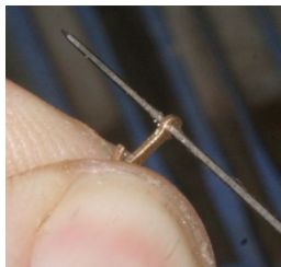
Ream the hole in the hook
