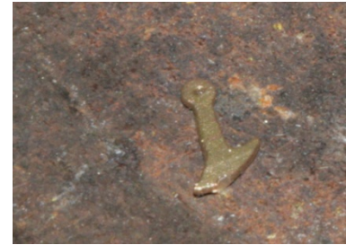
Remove a hook from the sprue and clean up the front face
